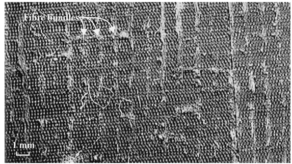
Fig. 5. Macrography of the heat sink after tests at 18 MW/m 2 (the defective tile was removed in laboratory).
